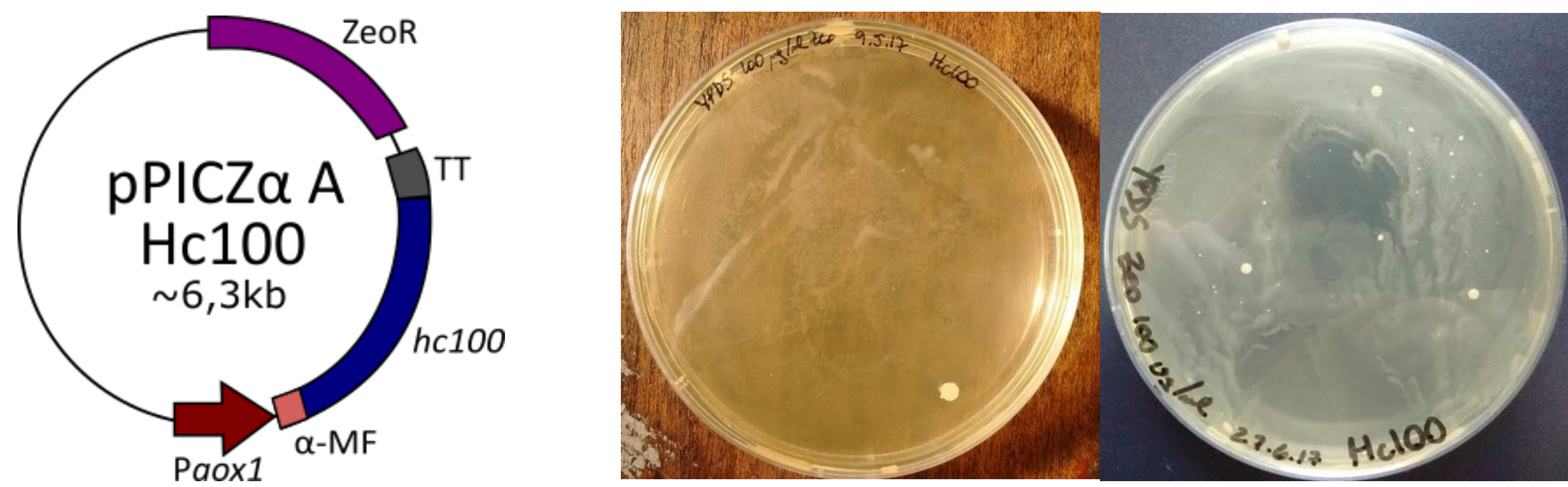
FIGURE 1. Pichia pastoris transformation. The gene that encodes for Hc100 was optimized for expression in P. pastoris and constructed with a secretory signal ( \alpha -MF) and a polyhistidine-tag. This construction was under the control of the methanol inducible promoter aox1 in the plasmid pPICZ \alpha A. Pichia pastoris X-33 strain was then transformed by electroporation and several colonies were obtained.
